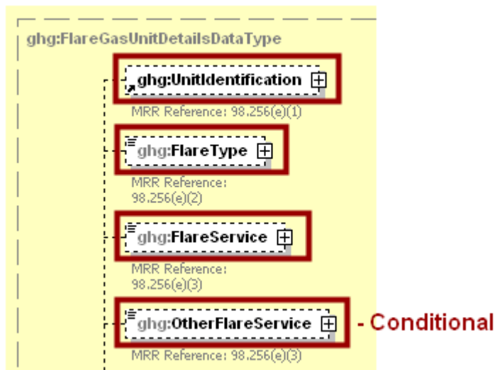
Figure 29 Flare Gas Unit Details Schema Diagram
