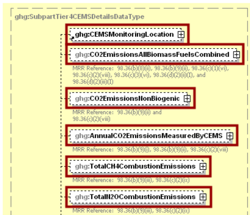
Figure 8 Tier 4 CEMS Location and Emission Details Schema Diagram
